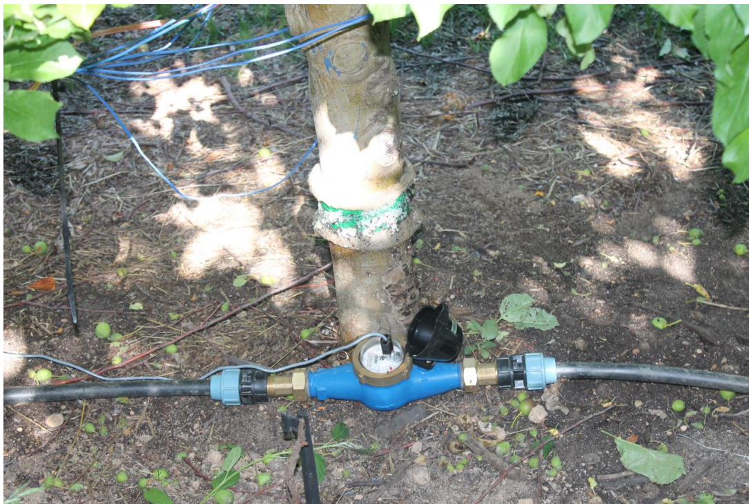
Fig. 3.5 Water flow meter measuring irrigation levels.
