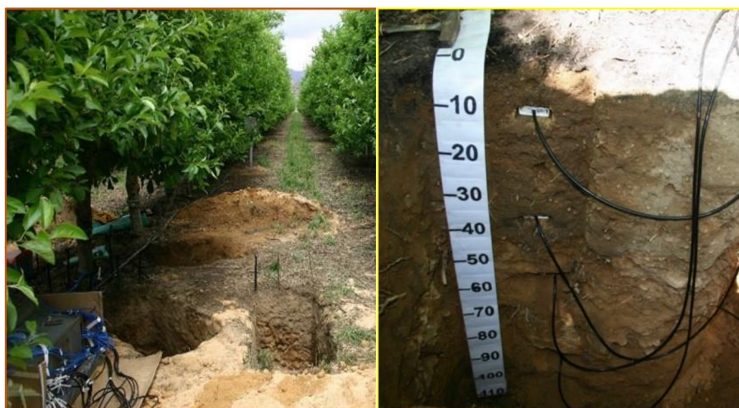
Fig. 5.1 Installation of CS616 sensors in the high canopy cover 'Golden Delicious' orchard at Kromfontein in 2014/15 in sandy loam soil at 150, 450, 750 and 1 050 mm depths. The measuring tape indicates centimetres.
