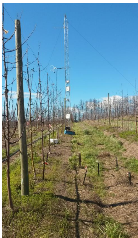
Fig. 3.9 Open path eddy covariance system deployed in a young apple orchard.
