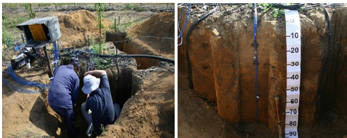
Fig. 3.3 Installation of CS616 sensors (black wires) and thermocouples (blue wires) in sandy soil in the low canopy cover ‘Golden Delicious Reinders’ orchard at Lindeshof in 2014/15. The measuring tape indicates centimetres.
