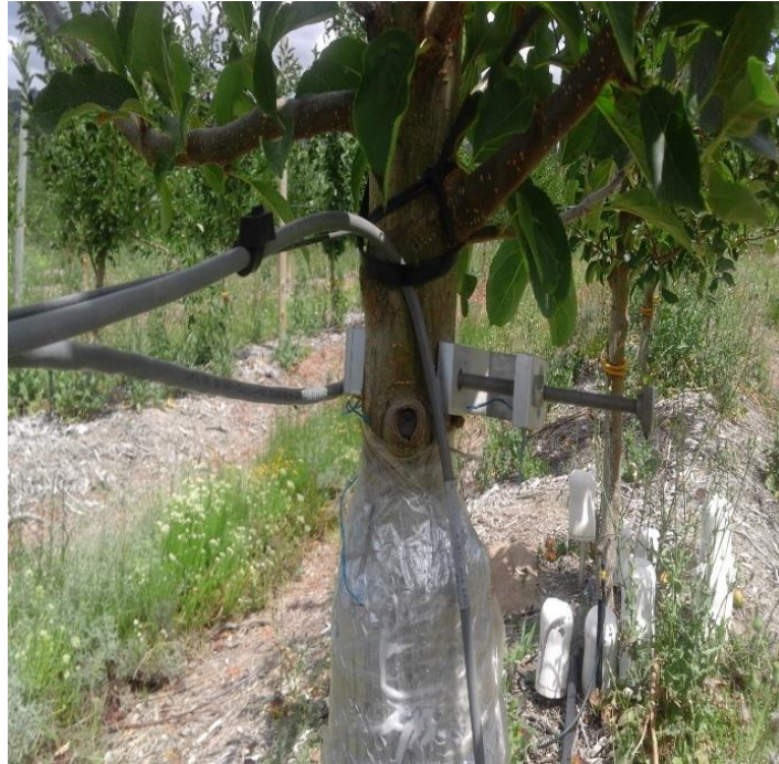
Fig. 3.6 The dendrometer used for monitoring stem diameter fluctuations.
