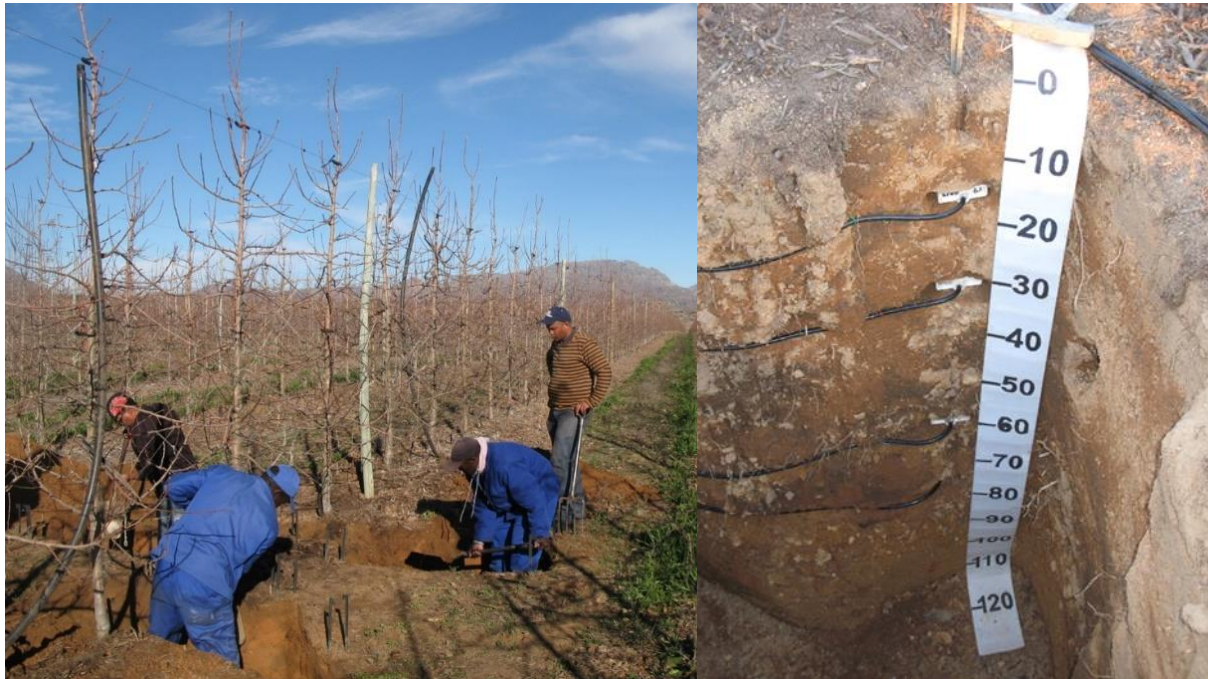
Fig. 4.1 Installation of CS616 sensors in sandy soil at 150, 300, 600 and 800 mm depths in the medium canopy cover ‘Golden Delicious’ orchard at Lindeshof in 2016/17. The measuring tape indicates centimetres.
