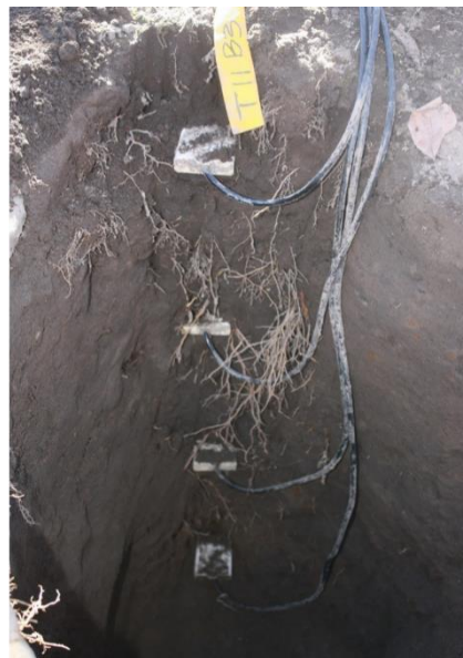
Fig. 5.2 Installation of CS616 sensors in 2015/16 in the high canopy cover 'Golden Delicious' orchard at Southfield (EGVV) in loamy sand to sandy loam soil at 150, 450, 750 and 1 1 00 mm depths.
