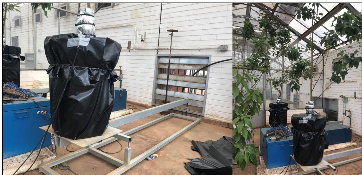
Fig. E2: Weighing lysimeters in the glasshouse used for the calibration of the TDP sensors in apple trees
