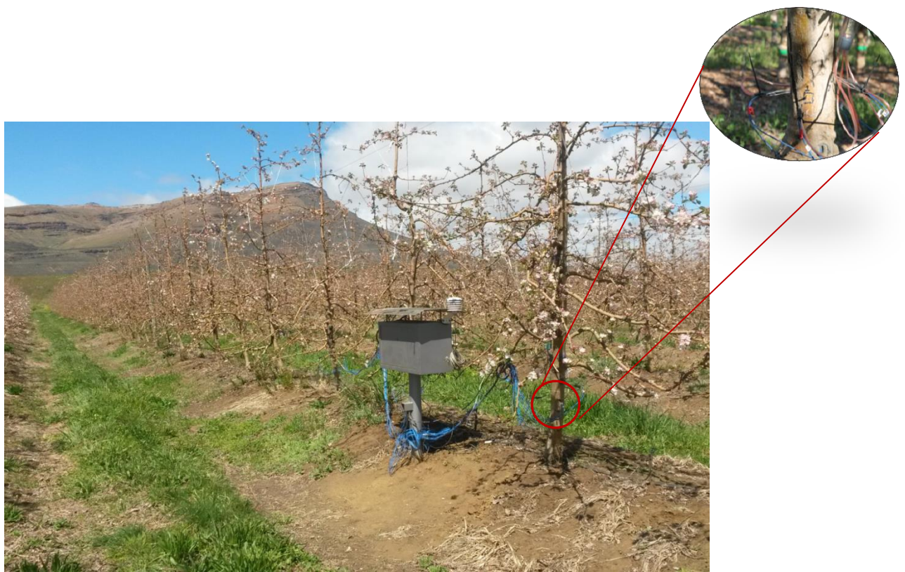
Fig. 4.3 Heat ratio method of the heat pulse velocity (HPV) sap flow technique. The grey security box contains the data logger, multiplexer, relay control module and battery. The insert shows a detailed view of the probes installed in the stems.
