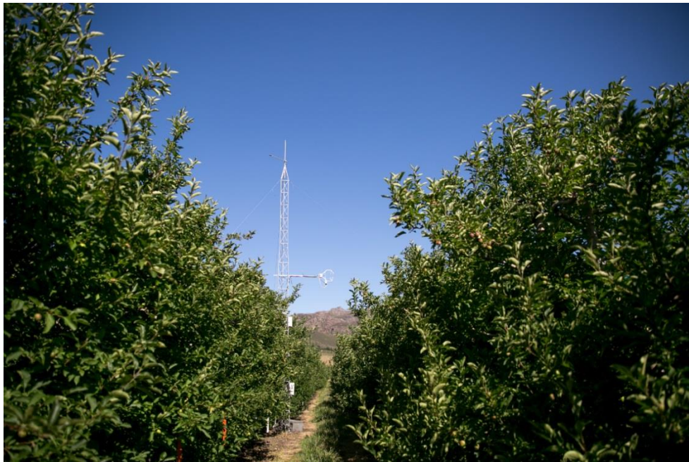
Fig. 5.3 Open path eddy covariance system monitoring evapotranspiration in a full-bearing 'Golden Delicious' orchard at Southfield farm in Villiersdorp.
